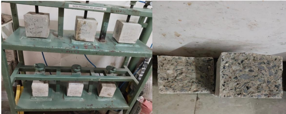
Fig 12: Water Penetration test on Bacterial Concrete
