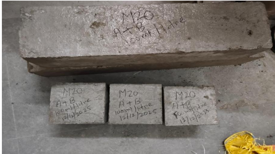
Fig 8: Casting of Bacterial Concrete
