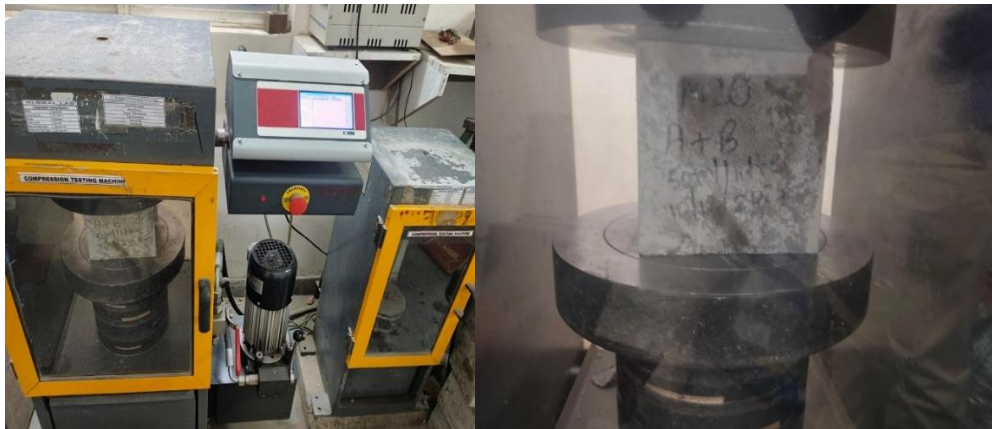
Fig 9: Compressive Strength test on Bacterial Concrete
