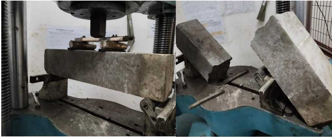
Fig 10: Flexural Strength test on Bacterial Concrete
