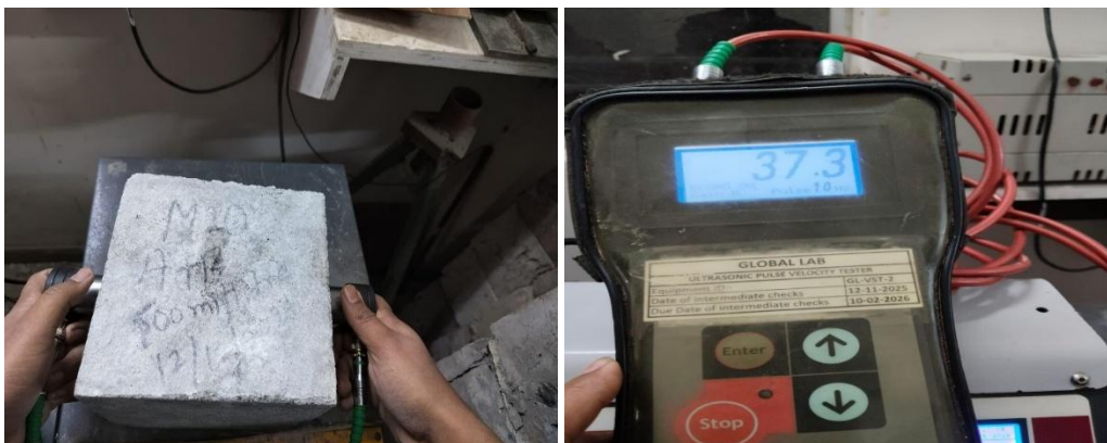
Fig 11: Ultrasonic Pulse Velocity test on Bacterial Concrete
